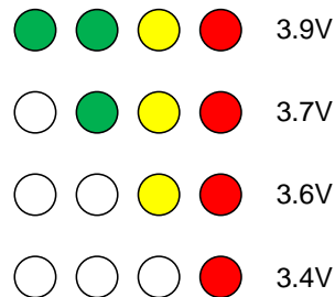
Figure 4: Battery voltage indicator states and corresponding voltages.
