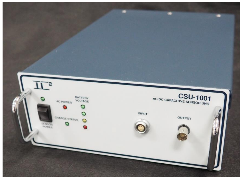
Figure 1: Photograph of the capacitive sensor unit.
